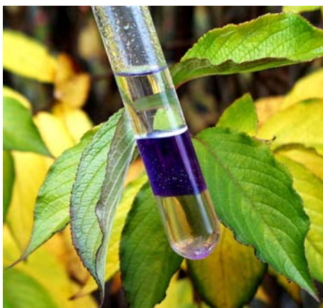
Figure D.3: Sustainable chemistry using Ionic liquids. The picture shows a test tube with a hydrophobic ionic liquid phase, a coloured water phase and a nonane phase. 8
